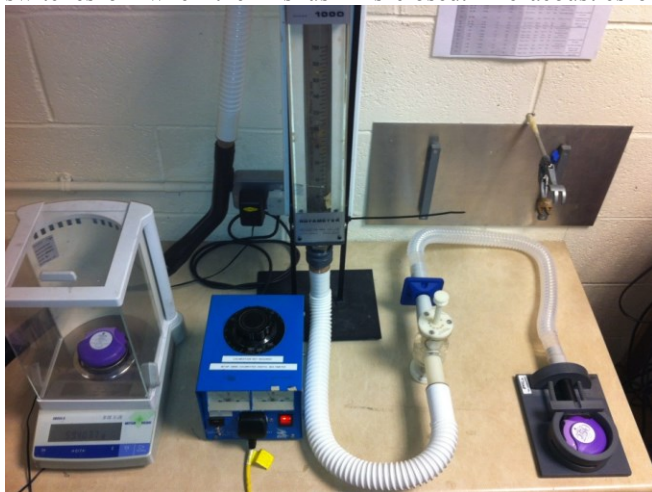
Figure 1: Test rig used to simulate inhalations in the in vitro experiment.
