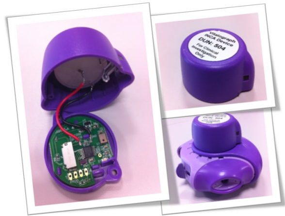
Figure 2: (Left) Internal components of INCA device, (Top Right) External view of INCA device and (Bottom Right) INCA device attached to Diskus™ inhaler.
