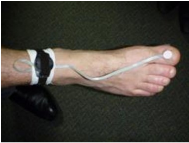
Figure 1. Placement of ankle accelerometer unit showing the auxiliary sensor on the superior surface of the great toe.
