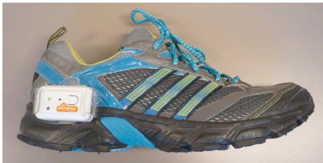
Figure 1: Sensor shoe setup – sport shoe with attached Shimmer sensor unit for gait analysis.
