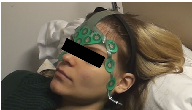
Figure 2. A screen printed electrode set applied to a human volunteer.
