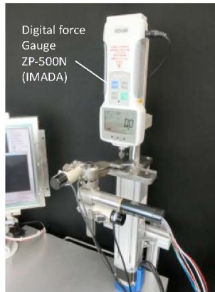
Fig.8 Force sensor calibration system using a digital force gauge
