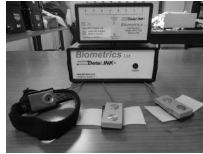
Figure 2: Biometrics system with electrodes and reference
