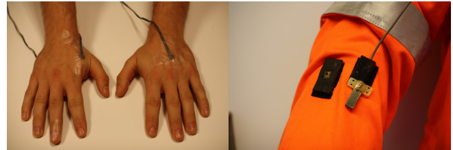
Figure 2 Location of YSI sensors on the hands (left picture) and location of HIH sensors compared to IsenseU Out (right picture).
