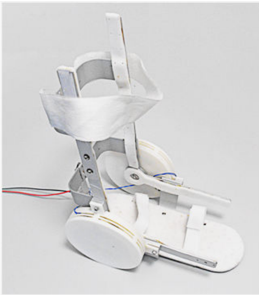
Figure 1. Mobilizer for the Ankle Joint. The two cylindrical housings on the two sides of the wearable device contain SMA-based amagnetic actuators that are compatible with MEG technology.
