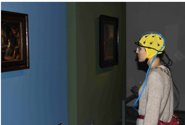
Figure 1. Gathering of the brain activity during the aesthetic observation of the painting "Young woman to the harpsicord" by G. Dou (1613-1675) at the art gallery "Scuderie del Quirinale" in Rome. Note the EEG cap and the eye-tracking device mounted on the cap for the monitoring of the eye movements. EEG and eye tracking data were stored on the portable devices brought by the subjects in a little bag near their hip.
