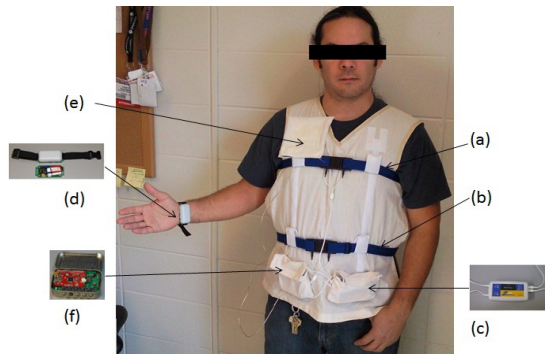
Figure 1. The PACT system, (a) Thoracic elastic band, (b) Abdominal elastic band, (c) electronic module for the portable Plethysmograph (RIP), (d) wrist worn RF transmitter of the PS system, (e) chest mounted RF receiver of the PS system, (f) data logger.
