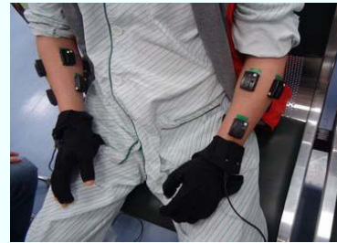
Figure 1. The placement of EMG electrodes and data glove wearing on both arm sides
