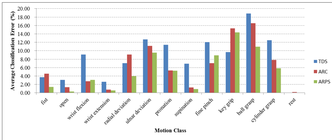
Fig. 6. Comparing average classification errors of specific motion classes among three sEMG features, TDS, ARC and ARPS.
