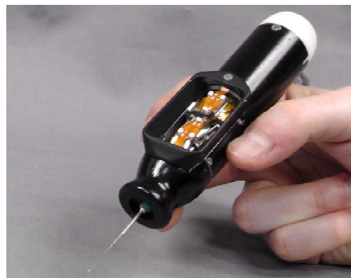
Figure 1. 6 DOF Micron. an active handheld micromanipulator.
