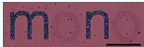
Figure 1. Synthetic control of graphene layers. Optical microscope image of graphene with differing number of layers. Letters 'o' are composed of ~6-10 layers and letters 'm' and 'n' 850 layers. Background is composed of bilayer graphene on 285 nm thick SiO 2 on Si substrate. Scale bar, 200 μm.
