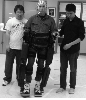
Fig. 1. A paraplegic volunteer controlling NeuroRex with his thoughts via our proposed EEG BMI interface
