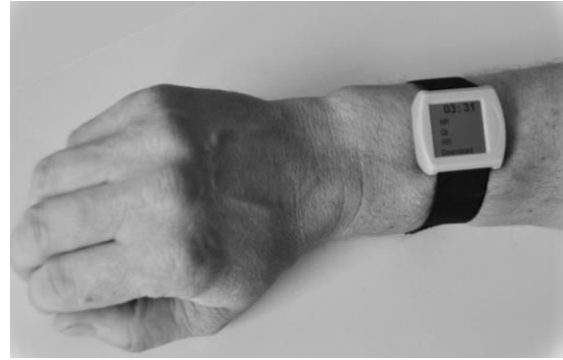
Figure 2. CSEM's proprietary wrist device for the estimation of RR intervals during night periods.
