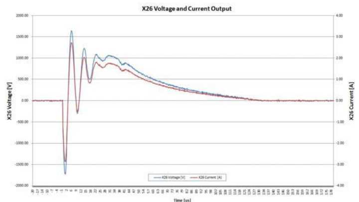
Fig. 1. TASER X26 CEW output for 600 Ω load.
