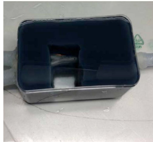
Fig 7: Carotid Phantom with agar-agar mimicking surrounding tissue
