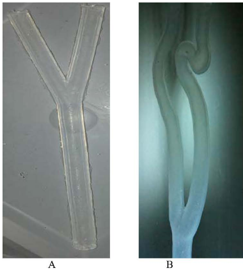
Fig 6: (A) Y-shaped transparent silicone model (B) Patient specific carotid transparent silicone model with siphon
