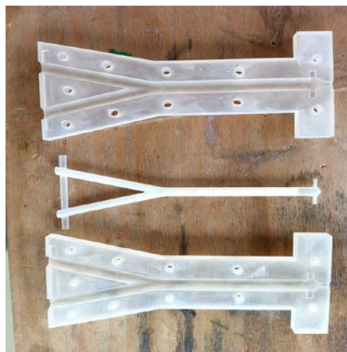
Fig 4: Rapid prototyping product of Y-shaped mold and core
