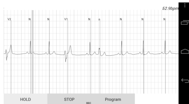
Fig.7. Results of classified ECG signal on the intelligent mobile phone.
