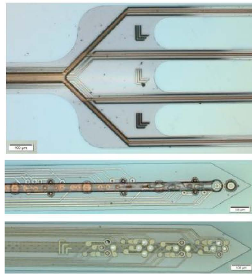
Figure 4. Images of three different multifunctional neural interfaces. The top image shows a probe with 4 separate shanks, where each shank has a fluidic channel. The middle image shows a single-shank design. The bottom image shows a single-shank design with a tetrode array. The top and middle images show top-down views of the neural interfaces (i.e. the fluidic channel is on top). The bottom image shows a bottom-up view of the neural interface (i.e. the electrodes are on top).
