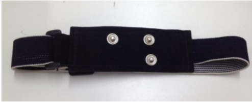
Figure 3. Conducting pad used as three dry electrodes
