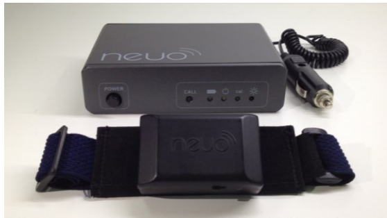
Figure 7. A portable wireless drowsy detection device
