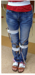
Fig. 1. System setup. Four inertial sensor modules were placed on human body segments, i.e. right thigh, right shank, and both feet.
