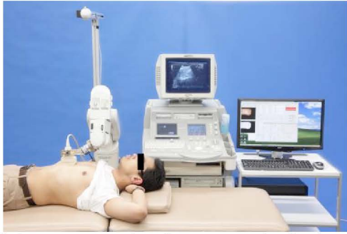
Figure 1: Autonomous scanning robot system consist of a robot attached with a camera and a force sensor, an ultrasound diagnosis device and a control PC
