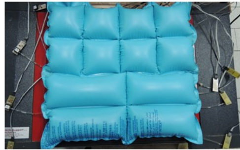
Figure 3. Designed cushion prototype with the sensors connected
