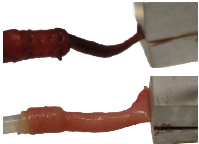
Figure 3. Rabbit esophagus (top) and pig esophagus (bottom) under suction with base tool.
