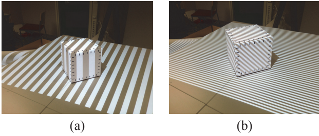
Fig. 4. A calibration between a camera, a projector and a referential object. Conventional Gray code pattern projection is utilized to calibrate a relative position and a posture between the devices and the referential object. (a) Vertical Gray code pattern projection. (b) Horizontal Gray code pattern projection.
