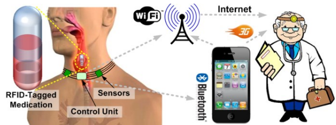
Figure 1. RFID-based Wireless and Wearable Event Detection and Adherence Monitoring System (WEAMS).
