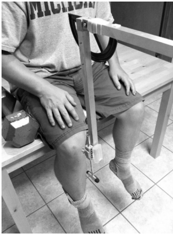
Figure 1. iPhone wireless accelerometer reflex quantification system. (mounted above and adjacent to the lateral malleolus)
