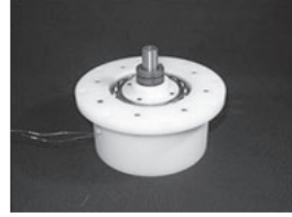
Fig. 2. Overview of a developed fast-response MR fluid brake
