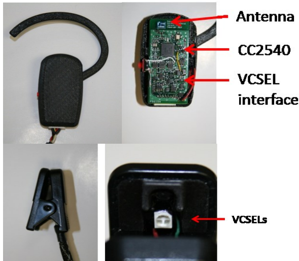
Figure 4. Prototype ear worn VCSEL based pulse oximeter. Top pictures show the electronics in the custom developed case. The bottom pictures show the modified ear clip with VCSELs replacing LEDs.
