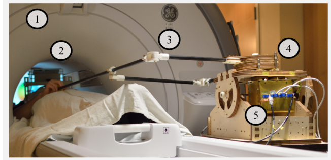
Fig. 1. Haptic fMRI. (1) Our novel three DOF fMRI-compatible haptic device, HFI, operating in a 3T MRI scanner. The subject uses mirrors to view a haptic simulation (2, painting) and interacts with it by manipulating HFI's four-bar linkage (3). Cable actuation (4) and RF shields (5) help minimize RF noise.
