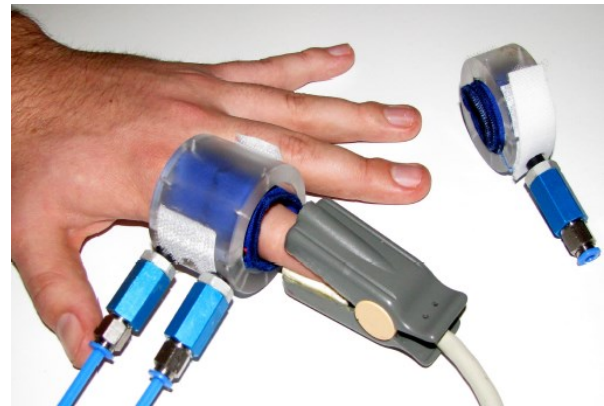
Figure 3. Artificial Pulse Generator and finger probe on a subject
