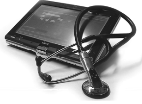
Fig. 2: Prototype of the DigiScope Collector system, composed by a tablet and an electronic stethoscope Littmann® 3200.
