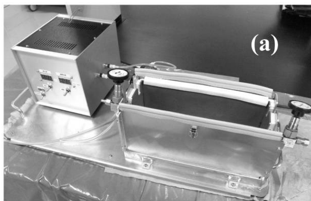
Figure 1. Outline of the system. The feature of the system is “double cold-trap”, which makes possible to detect only VOCs derived from the human body.
