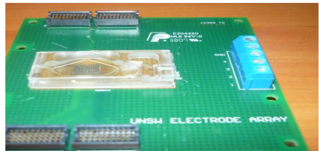
Fig. 1A: Electrode array board, with bath and connections to the data acquisition system.
