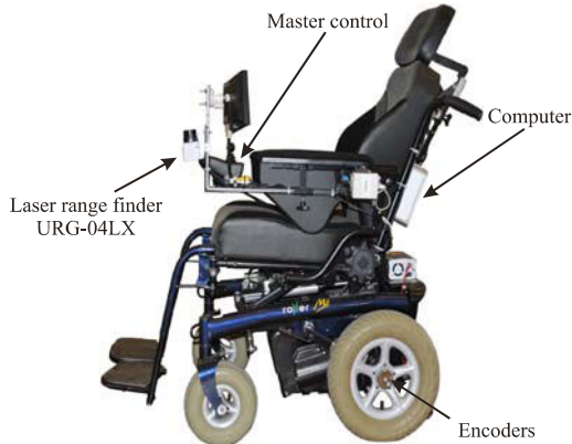
Fig.1. A prototype of intelligent wheelchair at the Centre for Health Technologies, University of Technology, Sydney.
