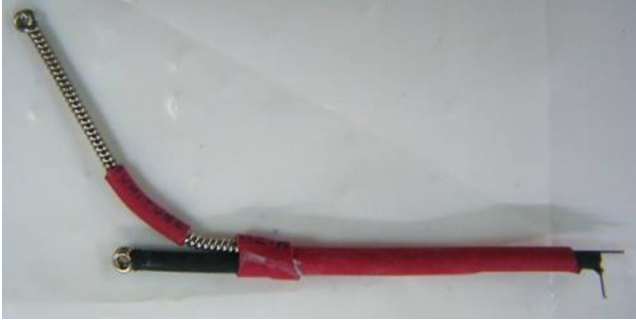
Figure 2. An assembled bipolar electrode for DRG stimulation in rat.
