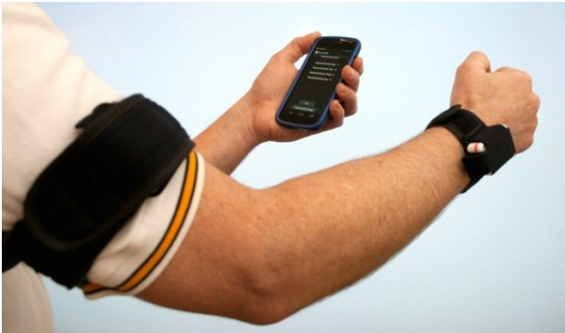
Figure 3. Motion Capture in progress. Shown are the MiMiC Application, Shimmer Kinematic Modules and the Kinematic Module Attachments.
