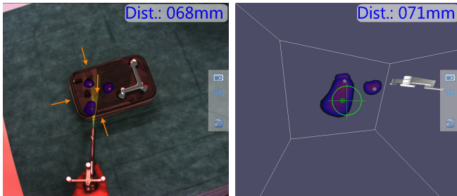
Fig. 3. Freehand SPECT visualization in two different modes: (a) as seen from the camera using augmented reality, (b) as seen from the probe tip in virtual reality mode. The arrows in (a) show the 4 scanning planes, 3 from the sides and one from top.
