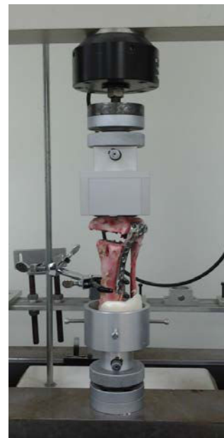
Figure 3. Testing model, providing vertical axial load pass through the center of tibial plateau and mechanical axis of tibia in the specimen
