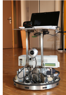
Fig. 1: Our telepresence platform is based upon Robotino by FESTO, which we have equipped with an additional wide-angle webcam and a laptop to facilitate remote interactions.
