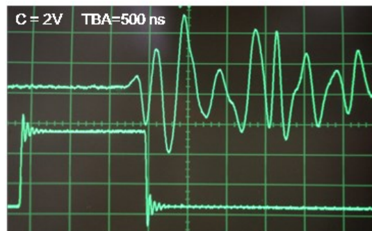
Fig. 5. The electrical ringing signal generated by the receiving transducer as a response to a single acoustic pulse. The control signal to the S/H circuit is shown on the bottom trace. The instantaneous value of the ringing signals is held at the falling edge of the control signal.
