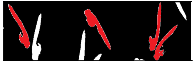
Fig 3. Perform Gaussian filtering with radius 6.0. Use global thresholding of 6 to isolate zebrafish embryo from background. Embryos in red indicate the ROI, whereas regions in white were discarded.
