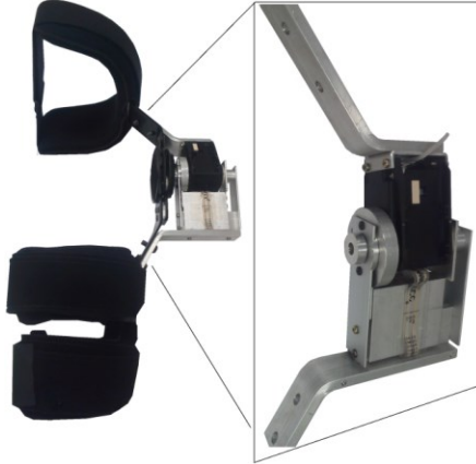
Figure 1. The RIAwAC attached to a mechanical orthosis designed to provide assistance/resistance in the knee joint.
