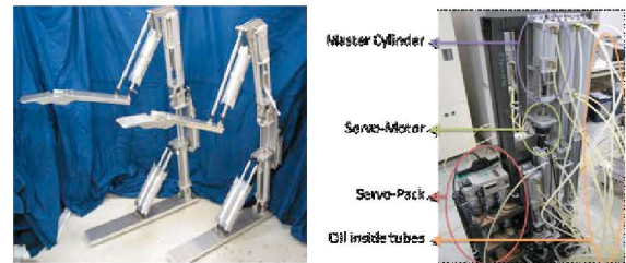
Figure 5. Body carrying attachable power assist device. Slave unit without the tubings (left) and Master unit (right). The dimensions of the master unit rack, including the 12 master cylinders and the Servopacks are 300 mm wide, 528 mm long, and 1370 mm high.
