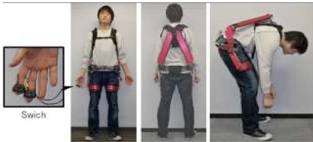
Figure 13. Overview of muscle suit developed
