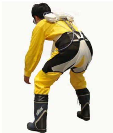
Fig. 1: Smart suit for 3-dimensional assist
