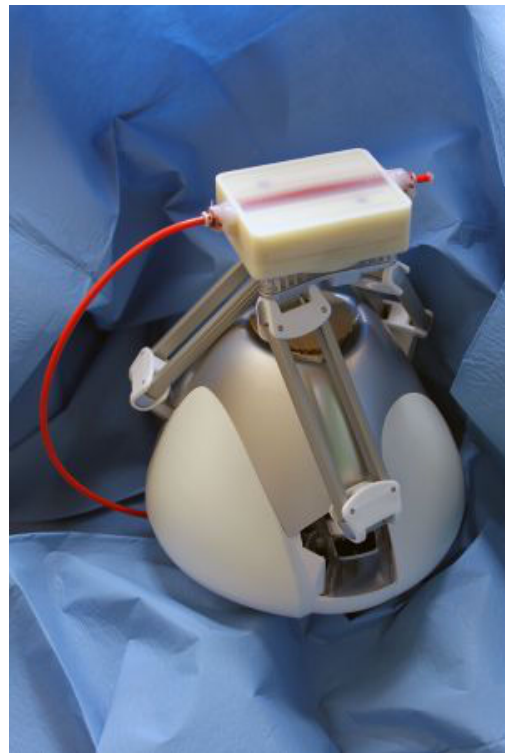
Fig. 8. PalpSim hydraulic pulse system
