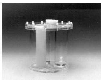
Figure 1. NEMA PET Phantom™ (NU2-1994)
