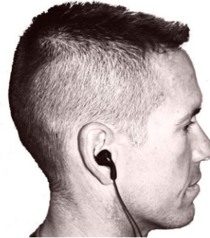
Figure 1. Example of the optical placement of the Valencell earbud integrated with physiological sensing using optical source and detector while exercising.
